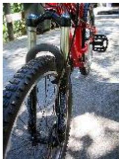
As far as frames in the Santa Cruz range go, the Heckler is something of a misfit. With a burly gusseted head tube, dropped top tube and 125mm of rear wheel travel from Santa Cruz's time tested mono-pivot suspension design, the frame is easily burly enough to be a 4X or dirt jumping machine but could just as easily be built up into a 12-13kg all day trail bike if that's "your thing".
